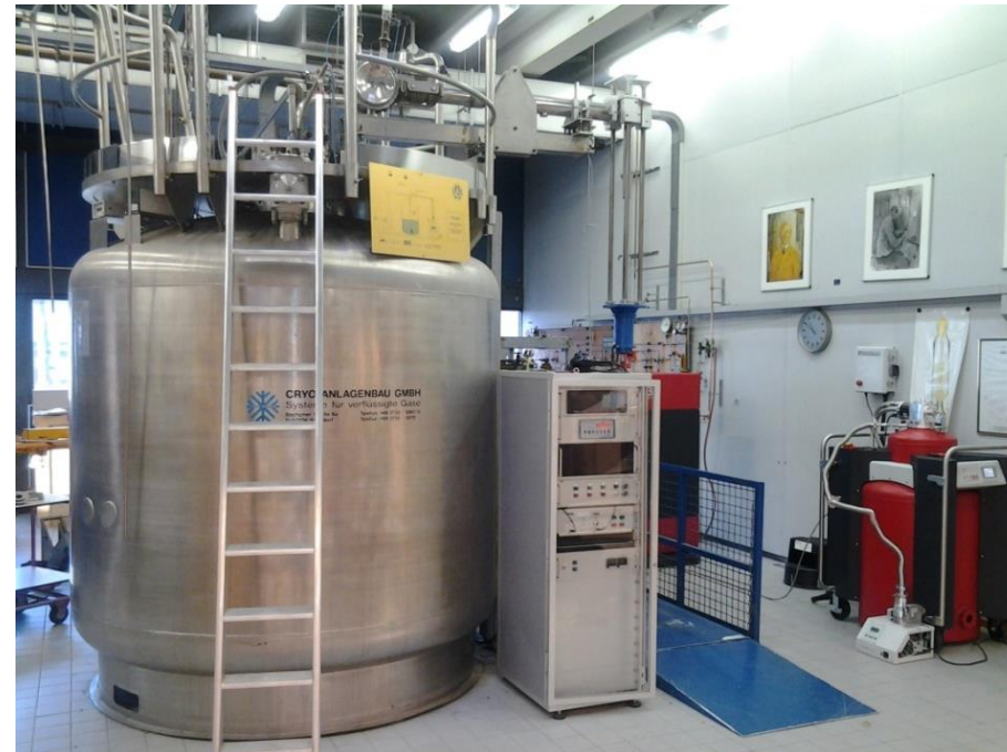
Uni Leiden: Big Dewar of industrial liquefier (left) and ATL160 (right)
